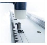
The assembly bushing is then driven in flush using a hammer.
