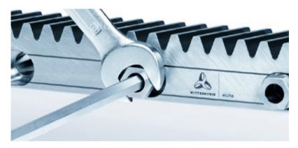
Previously, enormous effort was required to clamp racks to the mounting base using screw clamps. INIRA<sup>®</sup> clamping integrates the clamping device in the rack. The rack incorporates a mounting sleeve which is guided over the head of the fastening screw to ensure quick and ergonomic clamping.
