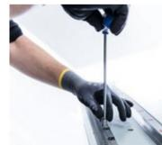
The assembly bushing and the assembly pin are turned in opposite directions until the bushing engages in the pin bore and then pushed in by hand up to the second marking.
