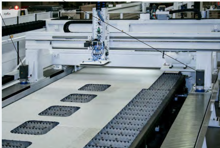
A rack-and-pinion system with four racks in a row is installed on either side of the portals.
